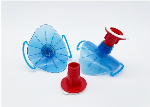
Filoform injection nipples and injection valves are used for injection joints. The injection valve is positioned on the wrap-around gauze by using the wrap-around tape. The injection nipple is placed onto the resin pack in order to enable an easy and smooth injection of the resin into the joint.
