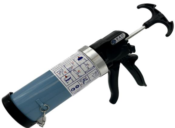
The new Filoform injection pumps are used to pump the resin under pressure ( $\pm 2$  Bar) into injection joints. The injection pump has a continuously variable piston displacement enabling an optimal flow of the resin into the joint.
